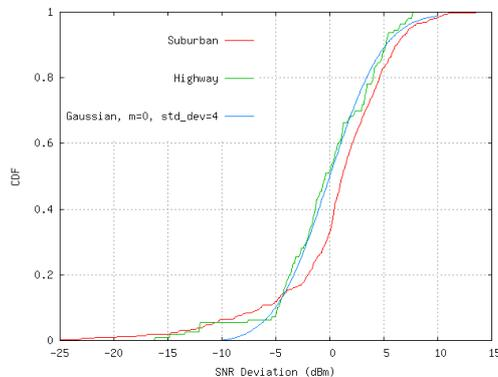
Fig. 6 CDF of gaussian distribution with mean = 0 and  $\sigma = 4$ ; and experimental distributions.
