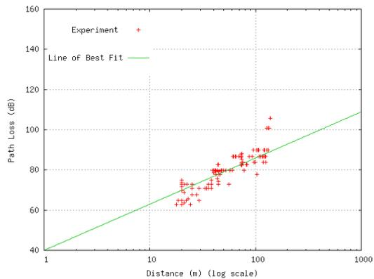
Fig. 5 Path Loss against distance for highway area with line of best fit of  $PL = 10 * 2.294766030 * \log_{10}(d) + 40.04$
