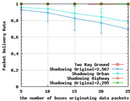
Fig. 10 Packet delivery rate for GPSR
