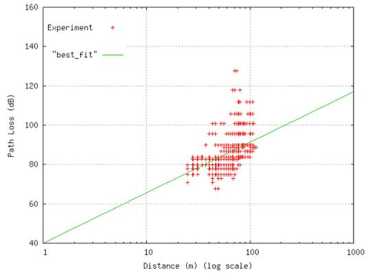
Fig. 4 Path Loss against distance for suburban area with line of best fit of  $PL = 10 * 2.566903837 * \log_{10}(d) + 40.04$
