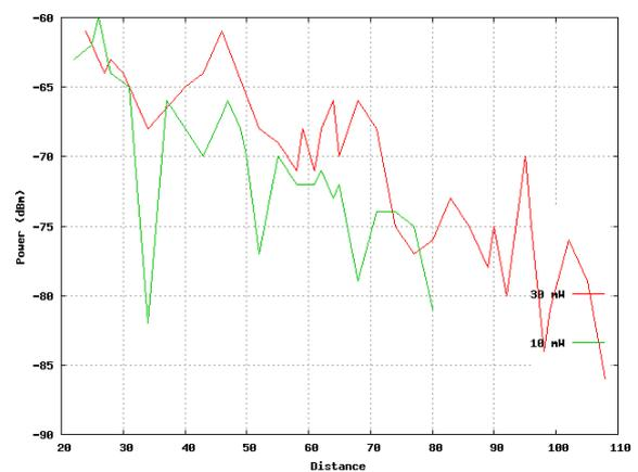
Figure 3: The effect of power variation on signal strength at suburban area using 1 Mbps transmission rate.
