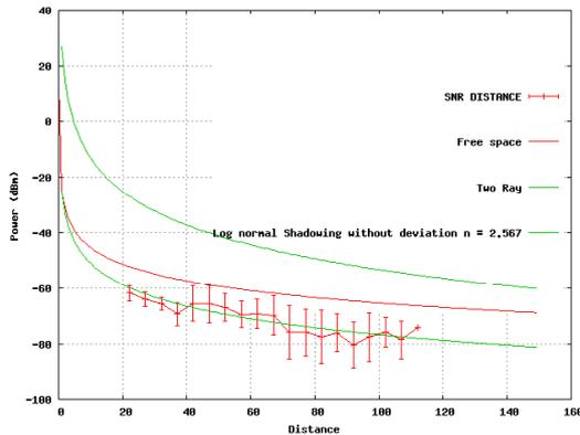
Fig. 8 Comparison between several radio propagation models with Experimental result at Suburban area.
