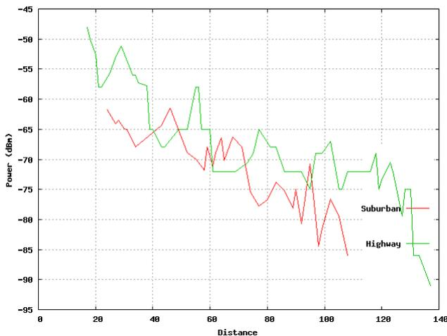
Fig. 2: The effect of location variation on signal strength using 30 mW power level and 1 Mbps transmission rate.
