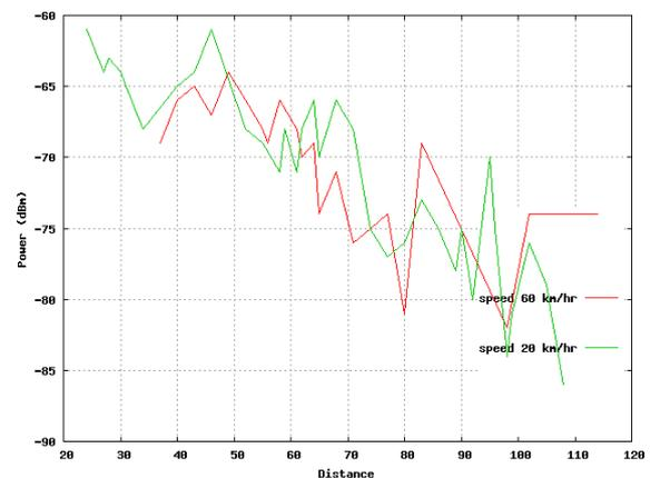
Fig. 1: The effect of speed variation on signal strength at suburban area using 30 mW power level and 1 Mbps transmission rate.
