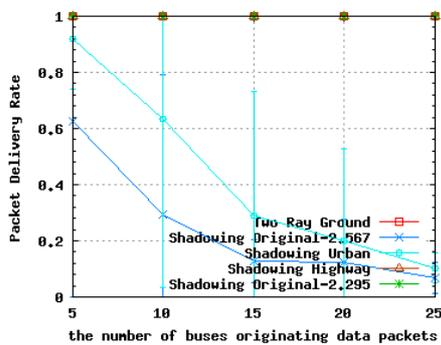
Fig. 11 Packet delivery rate for DSR
