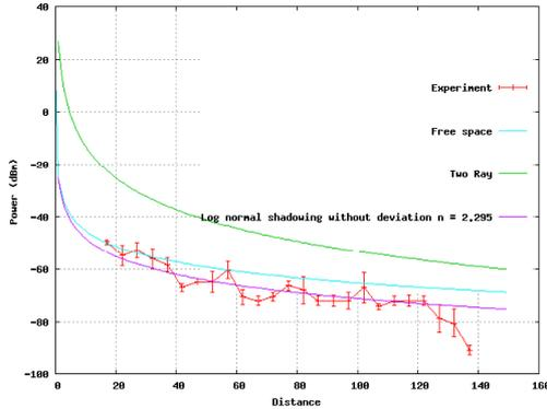
Fig. 7 Comparison between several radio propagation models with Experimental result at Highway area.
